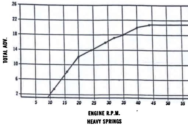
The curves listed above represent only approximate curves. Variations could be caused by a variety of things. i.e. lack of lube - rust, or other than stock advance weights.
